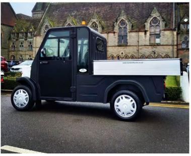
Height 1695 mm **Cargo Size** 1500x1300x265mm Length 3270 mm **Cargo Capacity** 500kg Width 1370 mm **Max Speed** 25 mph **Ground Clearance** 150 mm Wheelbase 2110 mm 8.5 KwH (Per 100km) **Tread** Front 1170 mm **Energy Consumption** Rear 1175 mm
